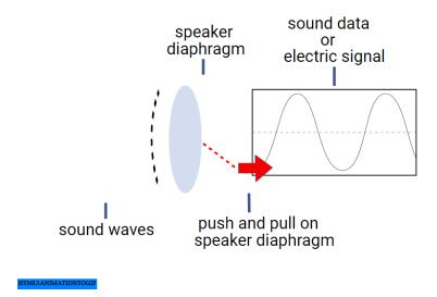
Fig. 4.13 How sound information turns into an electric signal, which then works with a magnet to push and pull on a <u>diaphragm inside a speaker</u> to create physical sound waves. Microphones do this process in exactly the reverse, the sound waves in the air make the speaker diaphragm go back and forth, making an electric current in the wire which gets measured and saved by the computer.
